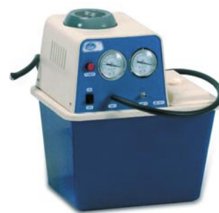
Water recirculation vacuum pump
